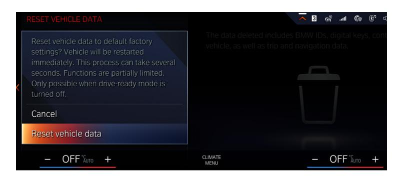
**4** The system will require a final confirmation. Select **Reset Vehicle Data** to confirm.
